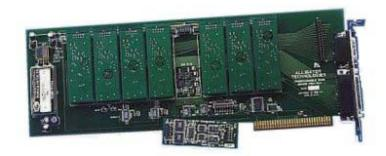
The PGA-16 is a 16-channel instrumentation amplifier with differential input, single-ended output, programmable AC or DC input coupling and pre-filter gain. The PGA-16 may be used as an input conditioner for any A/D converter or for our AAF-16 anti-alias filter card.
