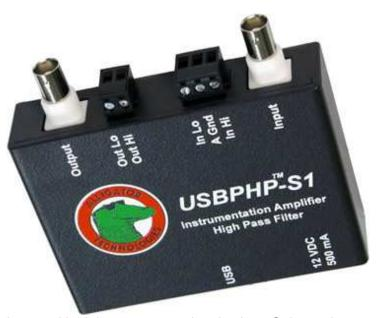
inputs with high-common mode rejection. Gain can be set at 1, 2, 5, 10, 20, 50, 100, 200, 500 or 1000. The USBPHP-S1 Instrumentation Amplifier provides an excellent common-mode rejection of 90 to 100 dB typical at high gains.
