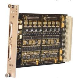
amplifier. The amplifier has an input voltage range of  $\pm 10V$  and is protected to  $\pm 40V$ . A common mode shield drive amplifier protects input signals.
